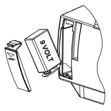
4.) Push the battery back into the battery compartment and replace the battery door.
